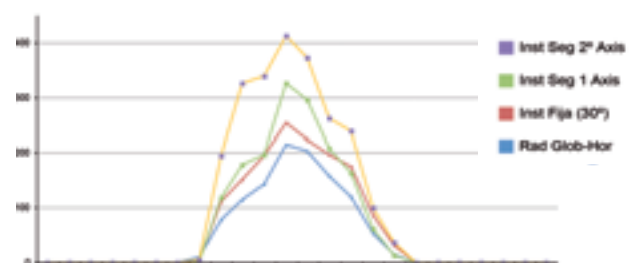
Comparison of the instantaneous power generated by solar panels mounted on different solar tracking systems.
