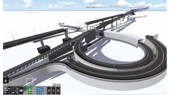
Example of the use of BIM in civil works: Américo Vespucio Oriente Project (Chile).
